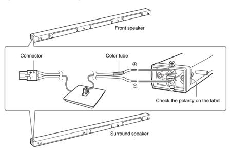
Insert the speaker cords into the speaker terminal of the speaker as far as they will go. Ensure that the cords are secure by gently pulling on them one at a time.
